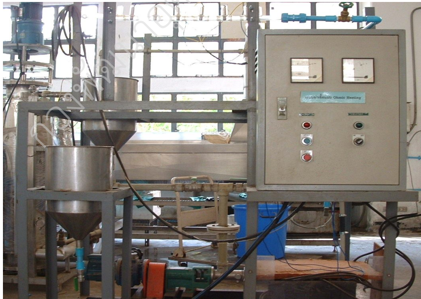
Figure 5: The Continuous Ohmic Heating System
